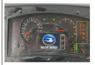
Once "wait to start" is no longer lit up in the dashboard it is ok to crank the bus.
